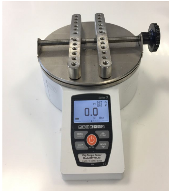
Figure 20. MARK-10 Model MTT01-12 digital torque meter
